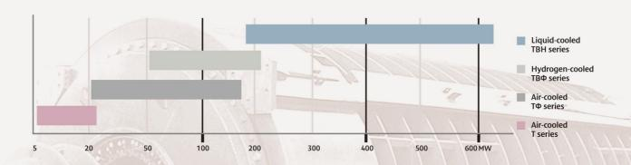
The generators supplied by "ELSIB" may be driven by steam and gas (heavy-duty or aeroderivative) turbines and create the optimum systems for central power plants, factory and city TPPs.
