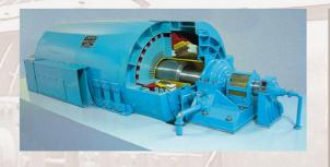
The generator rotor is cooled by water supplied and drained through a water-fed device located at the central part of rotor shaft. The supply of cooling water to the rotor winding is provided with the radial units of the water-fed device.
