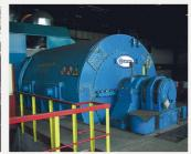
ydrogen is the superior coolant for the rotating electrical machines due to a combination of three outstanding properties – low density, high specific heat and thermal conductivity. The use of hydrogen allow to create compact, high effective, reliable and durable constructions.
